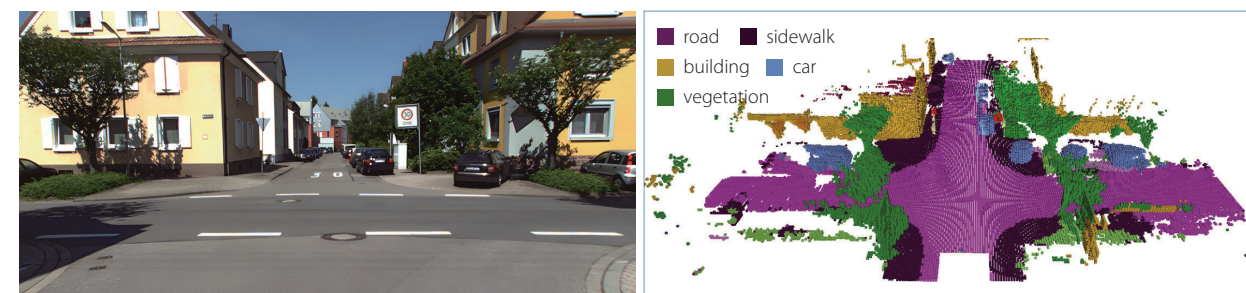
MARE (right) combines single-image semantic understanding and 3D reconstruction to estimate drivable space, overcoming long-tail object detection challenges and reducing autonomous driving costs.
